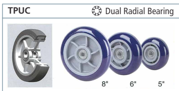
"Crowned TPU" TPUC -40° to 194°F 95A +/-3 TPU on Nylon Core
