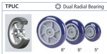
"Crowned TPU" TPUC -40° to 194°F 95A +/-3 TPU on Nylon Core
