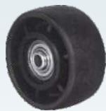
GFN -30° to 212°F 85D +/-5 Glass Filled Nylon
