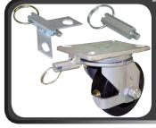
Position Swivel Lock converts a swivel caster to rigid. PSL can be disengaged to neutral position to allow for free swiveling action. The spring loaded plunger is hand operated to fit into slots in the swivel raceway. Can be purchased pre-welded to top plate or with wings that secure **PSL** to plate when mounting bolts to the top plate.
