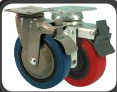
Double Locking Brake mechanism engages a positive braking action on the tread surface of the wheel, while simultaneously locking the swivel raceway in any position. Plastic pedal resists rust and corrosion in wet environments. Available in stainless steel.
