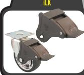
iLOCK™ is a precise eight position directional and wheel lock that provides perfect security. It engages with absolute precision and is available as a customizable one, two, three or four position lock. Engages with as little as 15 lbs of pressure and won't disengage at load with capacity of up to 1200 lbs. Brake pad adds extra security to harder wheel surfaces. Constructed of non-corrosive proprietary engineered thermo plastic. Virtually maintenance free.
