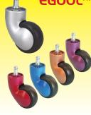
Egool<sup>TM</sup> is new addition to the Algood Ideal for store fixtures and institutional & food service equipment. Egool<sup>TM</sup> is available in a standard silver finish, with a 67mm diameter Polyolefin wheel and a 437Sx7/8 friction stem. It is available in swivel only, no brake. Weight capacity is 75lbs.
