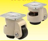
This die-cast aluminum levelling caster allows for moving heavy equipment. Once the equipment is in place, there is an adjustment knob in the back that is turned which brings down the foot or pad, lifting the wheel off the ground to prevent rolling. The foot is raised until the unit is level.
